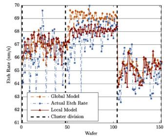
Fig. 7. Example etch rate estimates from global and clustered models using EP data as input.
