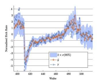
Fig. 10. Best etch rate estimates using windowed GPR model with window length 70.
